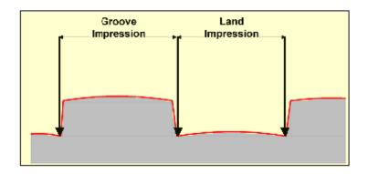
It may be necessary to measure several of the suitable land and groove impressions in order to obtain a reliable measurement. At a minimum, one land impression measurement and one groove impression measurement, recorded to the nearest thousandth of an inch, shall be recorded in the notes for each bullet. Methods may include the Leica Application Suite Measurement Module and the air gap method.
