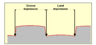
All suitable land and groove impressions shall be measured and their average measurement, recorded to the nearest thousandth of an inch, shall be recorded in the notes for each bullet. Methods may include the Leica Application Suite Measurement Module and the air gap method.
