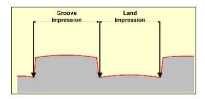
All suitable land and groove impressions shall be measured and their average measurement, recorded to the nearest thousandth of an inch, shall be recorded in the notes for each bullet. Methods may include the Leica Application Suite Measurement Module and the air gap method.
